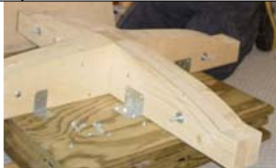
Figure 4 - Motion platform showing rocker and 2-way sliding base
