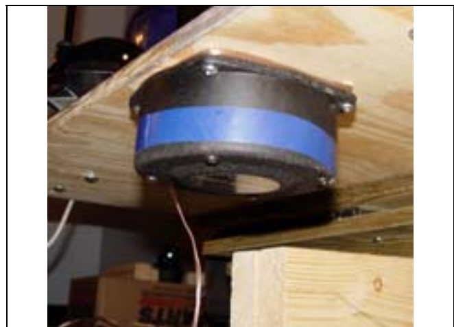
Figure 2 - Bass Shaker installed underneath the motion platform
